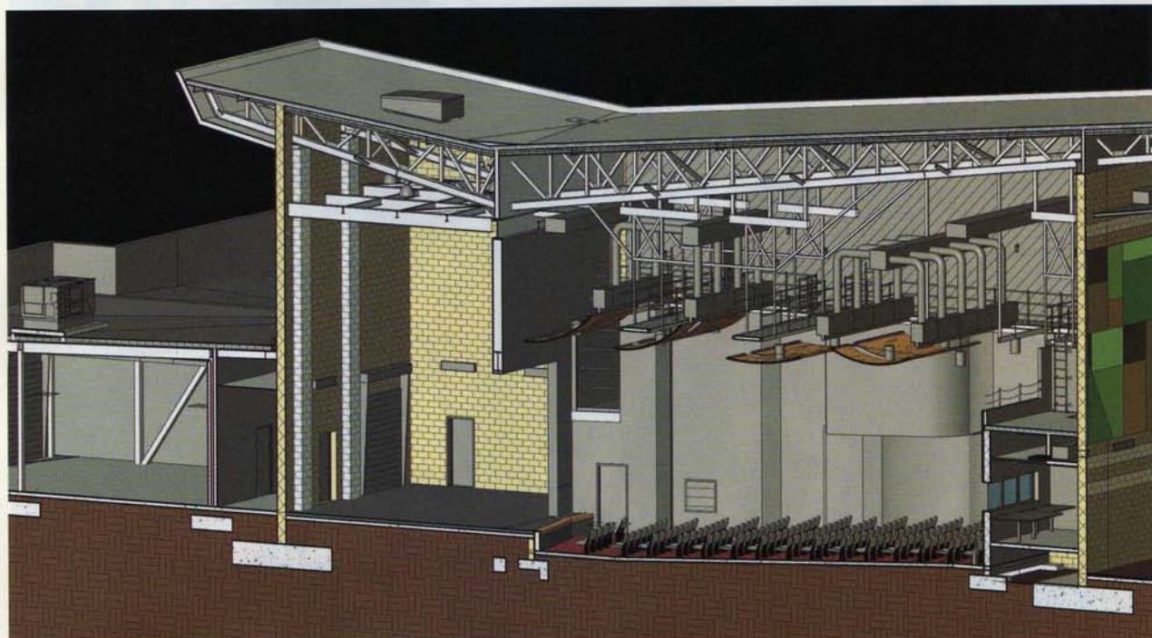
The Oxnard Community College Performing Arts Center is using BIM for its structural and mechanical equipment.
